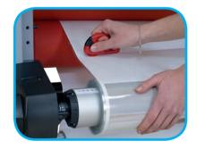
In order to protect the laminating rollers from unsafe operation when not using a proper cutter, a safety cutter is delivered with the machine. The quality of your lamination job and your investment are preserved for years.
