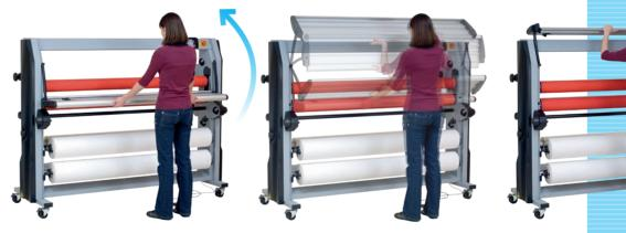
The feeding tray pivots upwards leaving a full and secure access to the machine when loading the film. In upper position, the driving motor is shut, preventing the operator from any injury during the operation.
