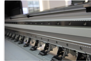
Aluminum beam& dual linear guides
